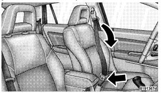
**Inserting Latch Plate Into Buckle**
